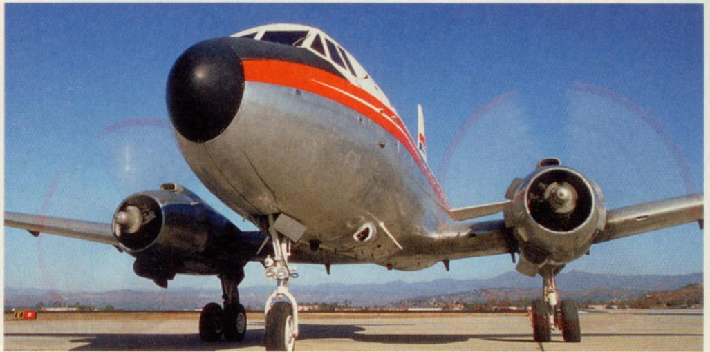
**The 404 is a big bird: 44,900 lbs max takeoff weight, and 4,100 total horsepower.**
